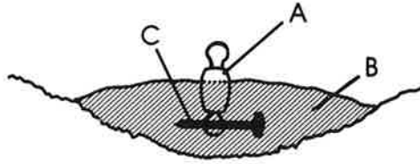
FIG. 2. Stainless steel fishing swivel (A) cemented on the rock substrate. One end of the fishing swivel was embedded in the cement (B) and anchored with 2.5-cm steel nail (C).
